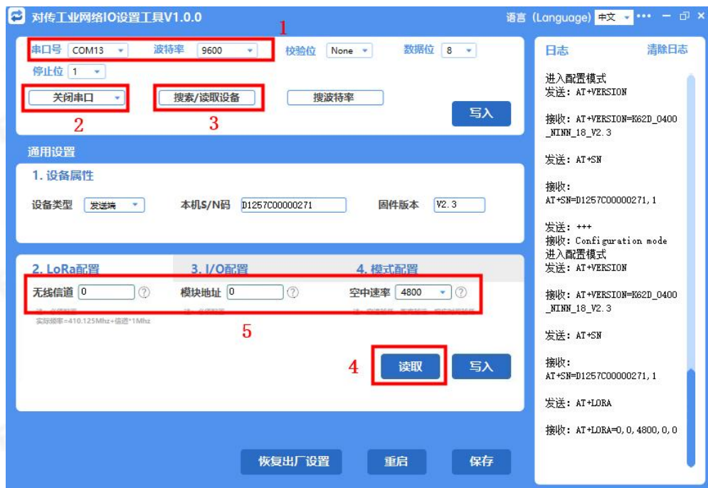
Figure 4-9 LoRa parameter reading
