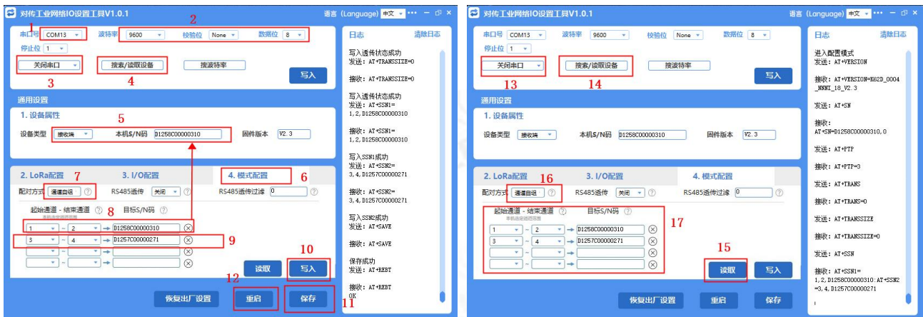
Figure 4-26 D1258C0000310 Receiver configuration writing steps
