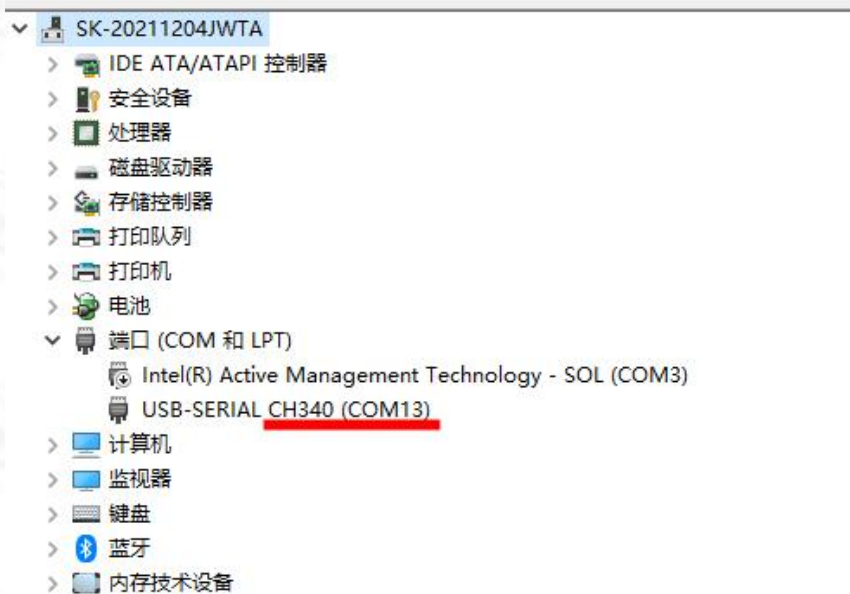
Figure 4-8 Computer port of USB to RS485 module
