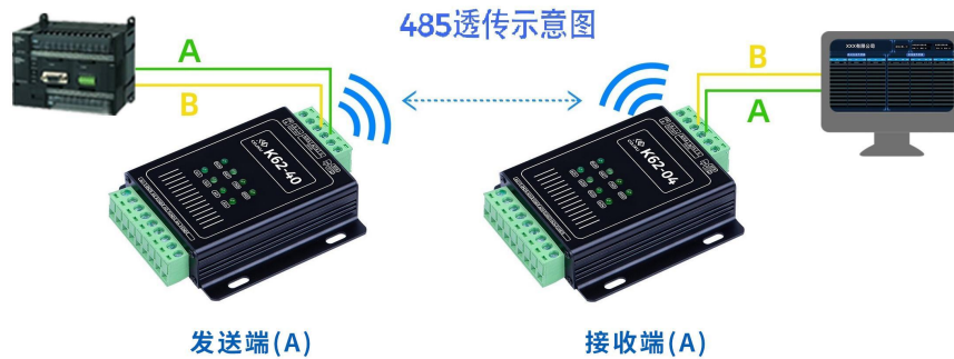
Figure 4-20 Schematic diagram of 485 transparent transmission
