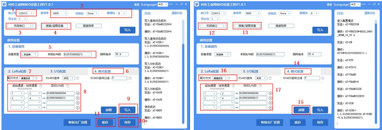
Figure 4-24 D1257C0000271 Sender configuration writing steps
