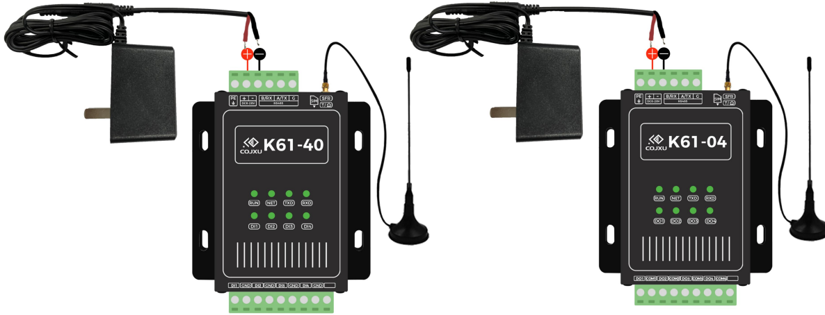
Figure 2-2 Connecting the antenna and power
